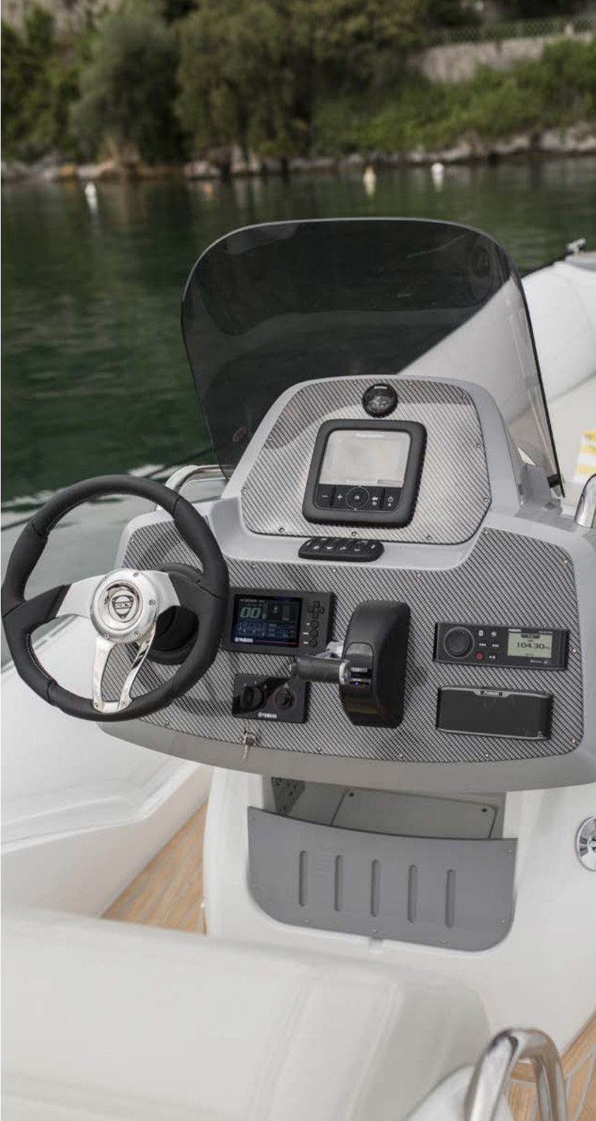
Central console with windshield, stainless steel handrail and glove compartment
