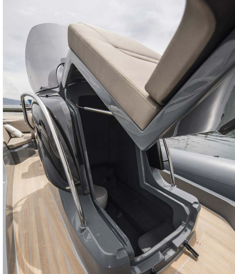
Toilet under console
